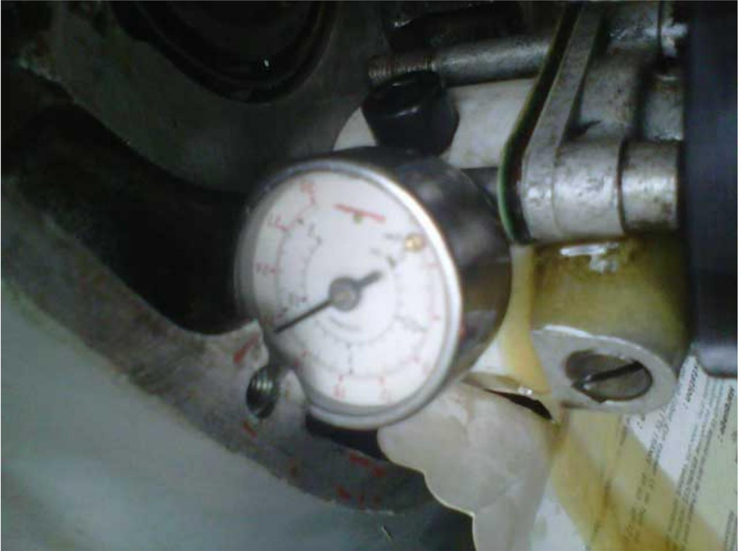
With the screw used to adjust the pressure flush with the pump's corpse the pressure fluctuates around 1,5 bar (22 PSI).
