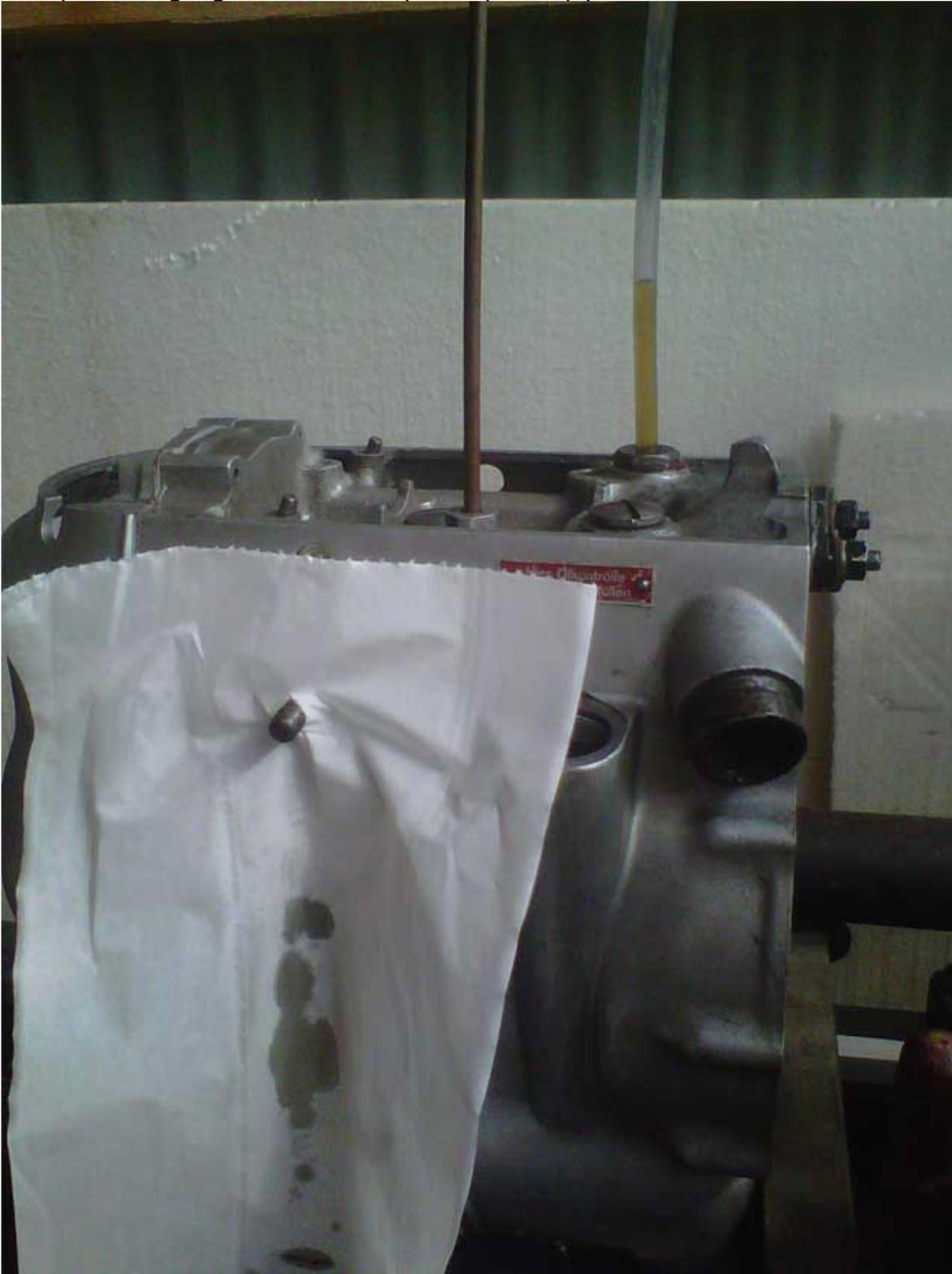
One can see that, once the circuit is filled, the crankshaft splashes on the paper. That was done at 125 rpm. The pressure stabilizes at around 15 millibar (0.2 PSI) after some time:
