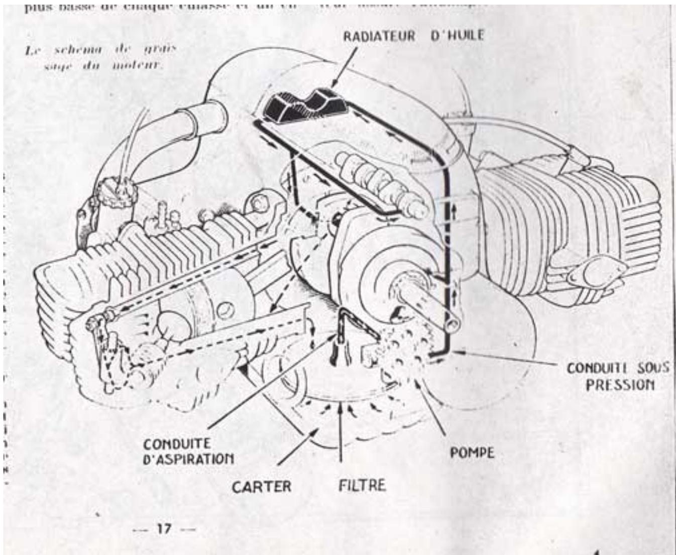
Oil is taken in the sump through a strainer which is a simple steel mesh. (I changed this mesh I found too large for a finer stainless steel one). The figure above mentions « filtre » (filter) which is for the KS601 engine depicted, not existing on my KS600.
