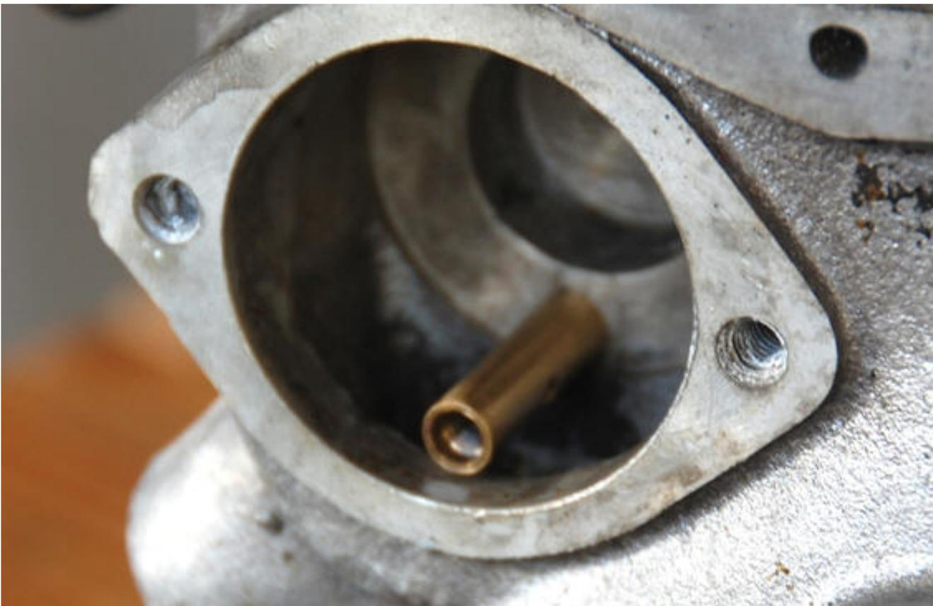
It is made of bronze and force fed in a 6 mm hole coming from the pump output. It can be removed with the aid of an M5 screw and nut:
