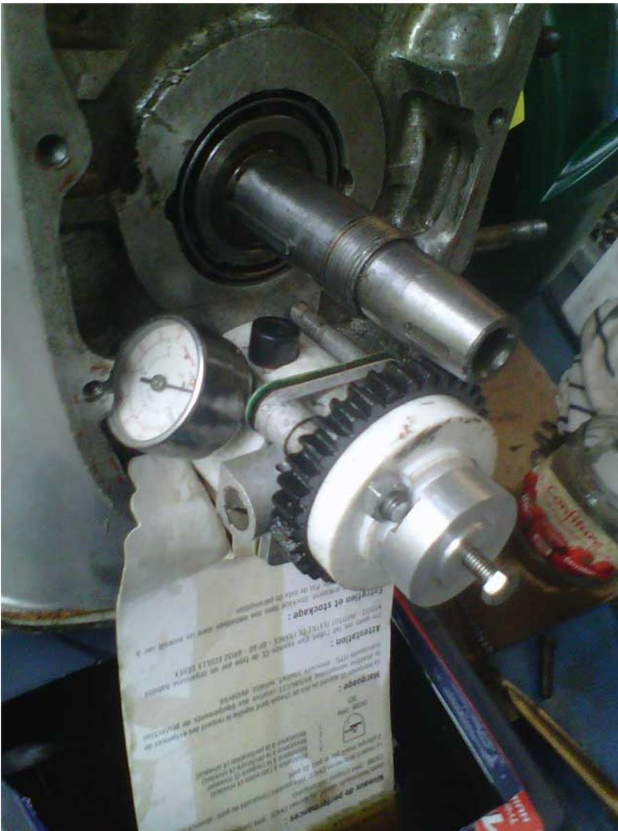
This spacer allowed me to insert my gauge in the pump output before the limiting jet. The cardboard is there to help the oil from the discharge valve to reach the can under.
