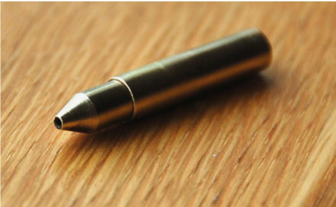
Oil enters the jet by the 1 mm hole on the left. The cone shape is to avoid dirt clogging the small hole.
