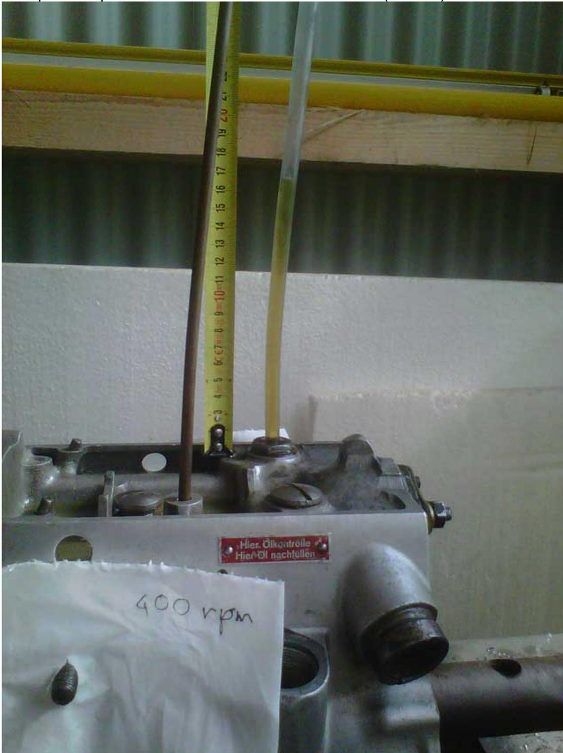
400 rpm here but the oil level is independent of the rpm because as soon as the pump's discharge valve is opened the output pressure of 1,5 bar is constant. This happens well under the engine's idle rpm.
